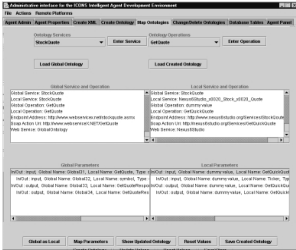
Figure 10. Diagram of the ontology being mapped to a global ontology. Global ontology is on the left and the ontology just created is on the right
